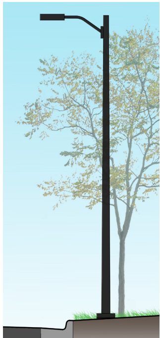
Roadway light (30' height)
