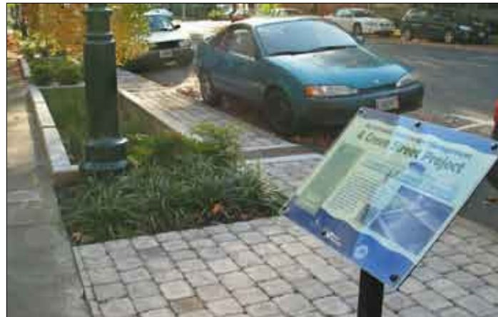
Figure 37: Utilize pervious pavers to encourage permeability.
