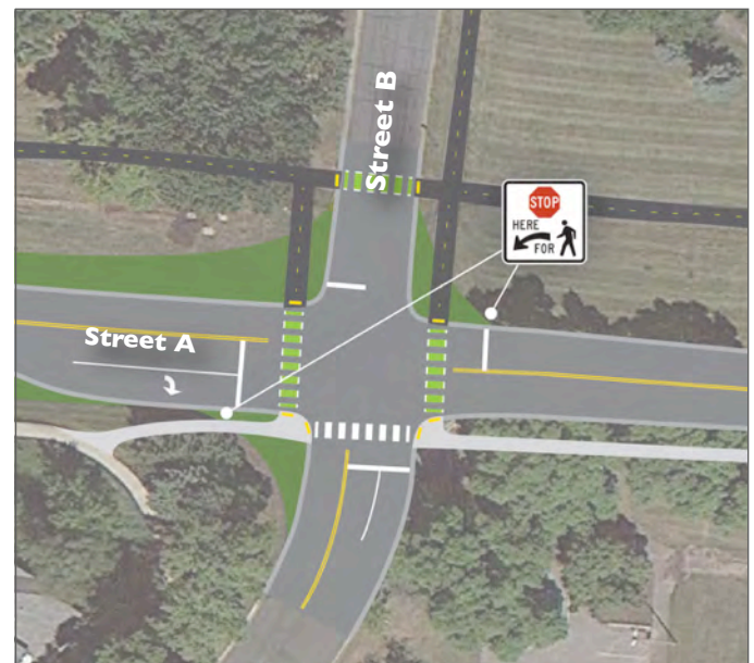
Alternative 1: Reducing the turning radii, removing the right turn slip lane, and adding high visibility crosswalks as well as additional sidewalk and shared-use path elements would help to enhance pedestrian and bicyclist visibility and facilitate overall connectivity.
