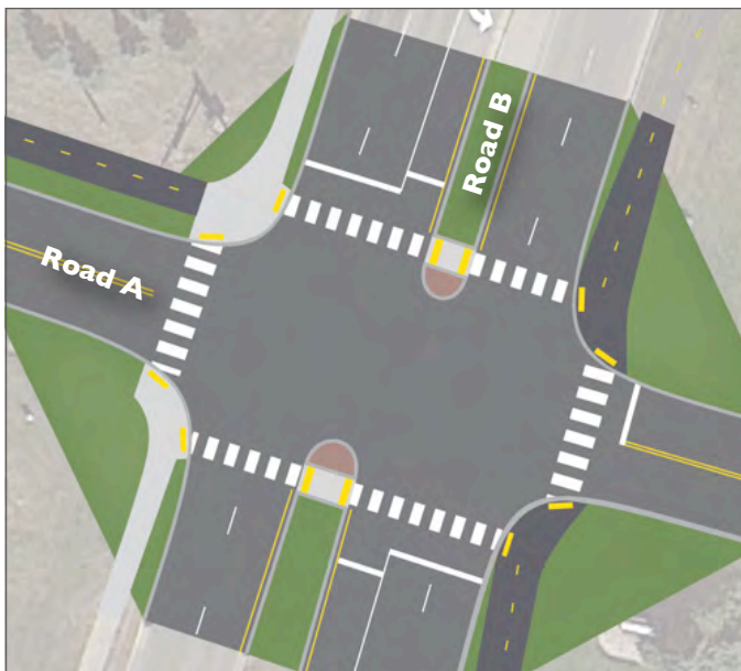
Alternative 1: High visibility crosswalks, refuge islands, and vehicle stop bars are added to increase the comfort for pedestrians.
