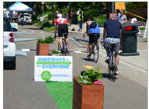
Special events offer a chance to take part in "tactical urbanism" and try out infrastructure treatments before they become permanent. Here, users try out a "pop-up" protected bikeway treatment at an Open Streets event.
