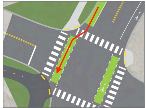
Green paint can help direct bicyclists and alert motorists when there is a transition from an on-street to an off-street bicycle facility.
