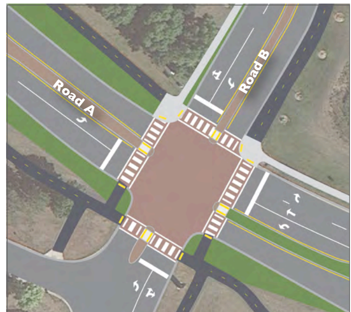
Alternative 2: Eliminating lanes allow corners to be brought in and further reduce the total crossing distance.
