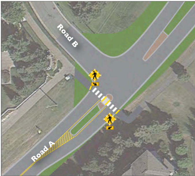
Alternative 1: Removing the left turn lane on the west side of the intersection allows for the addition of a center median and a pedestrian refuge island. These modifications should help reduce motor-vehicle speeds at the point of the crossing and break up the total crossing distance for pedestrians.
