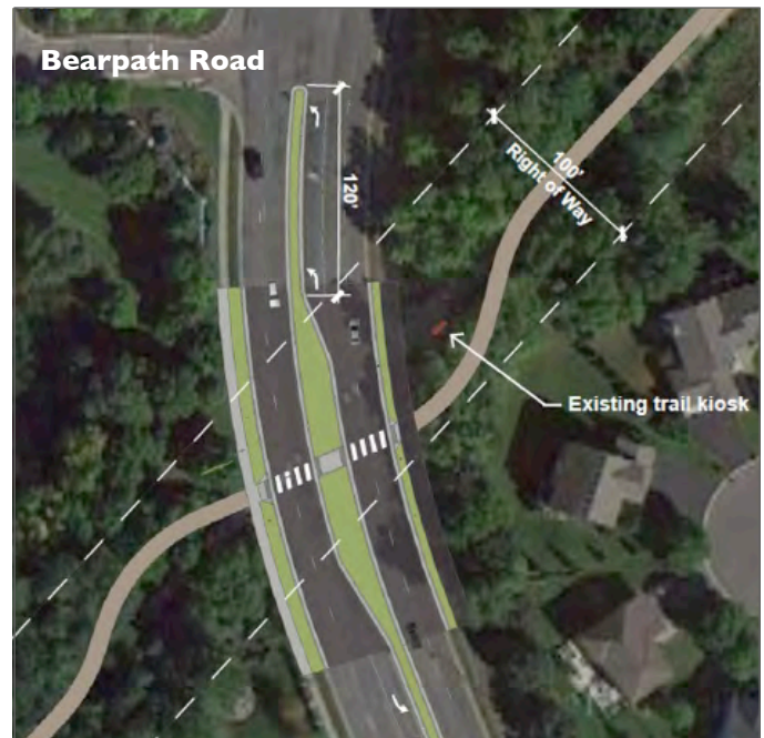
Proposed: Realigning the trail and shortening the left turn lane increases visibility and protection for those crossing at this location. Another potential element (not shown) is to add an advanced yield bar ahead of the crosswalk.
